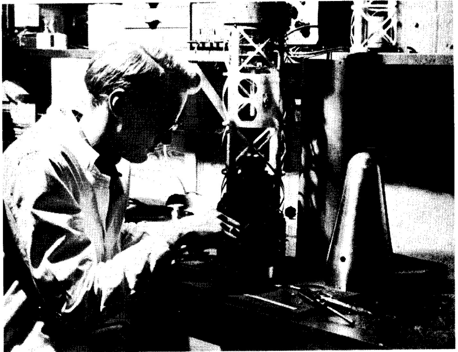
—Wide World Photo Instruments being installed in "Explorer" satellite. Two transmitters, one at top and one below in the sleeve, are to convey scientific information to tracking stations. Scientists hope to learn if it will be safe for human beings to venture into outer space.
